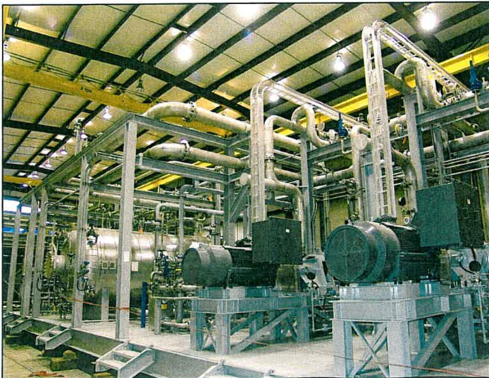
■ HC Piper's Series 5 VRUs are highly engineered units. The compressors on the packages start, stop and switch to bypass control automatically. The packages run without operator intervention, other than the periodic maintenance of the compressors' mechanical seals and bearings.
